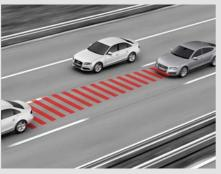
Adaptive Cruise Control with Stop&Go and Traffic-jam assist
